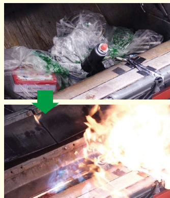
Cases of ignition of gas cartridges in collection vehicles [Source: NITE].
